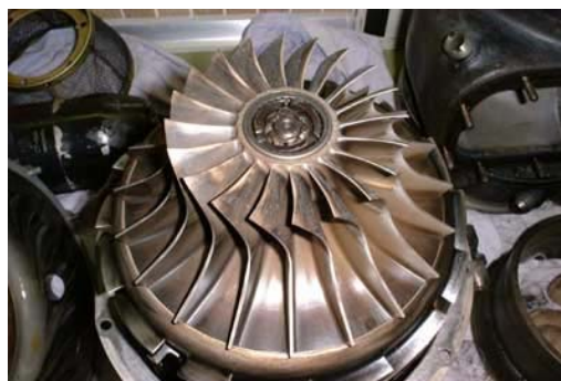
Figure 5-9 APU Compressor Rotor
