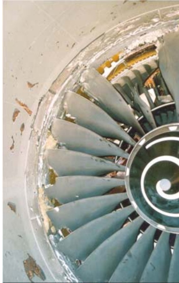
Figure 5-10 Actual field event fan blade release and damage to the trailing blades
